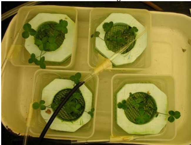
Figure 2. Hydroponics setup of Clover seedlings grown at various concentrations of \text{Cd}^{2+} .
